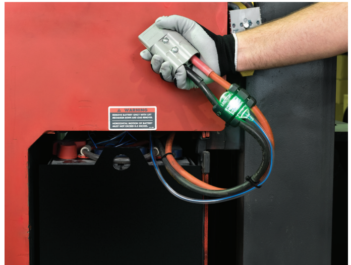
Blinking green LED indicates electrolyte level is good
